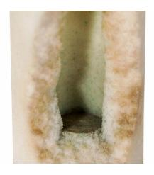
The inside of the filter is completely degraded and saturated with particles. The porosity is lost.
