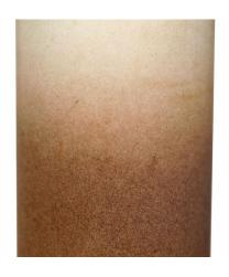
A photo micrograph of the filter element shows the rust particle contamination.
