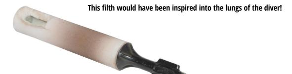
This is a MicroMaxx filter completely clogged and contaminated with oxide particulate after seven years of use.
